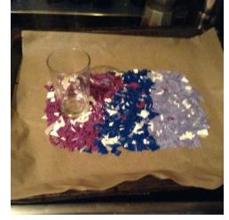
example, the plastic was cooled, flipped over, and placed back into the oven for molding purposes.
