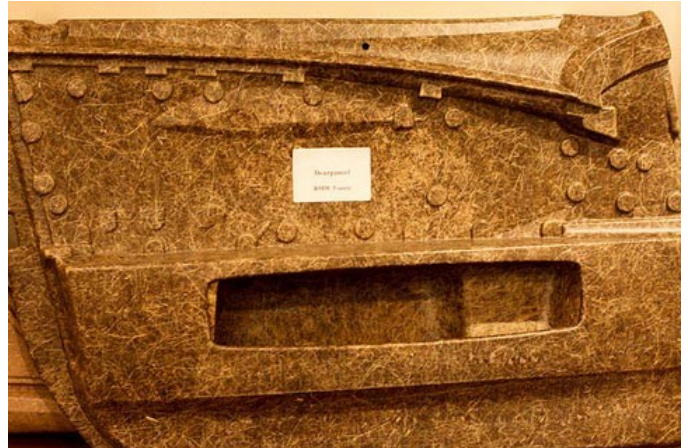
Figure 2: BMW i3 saves weight using hemp fibers. Hemp-based door panel in the car.
