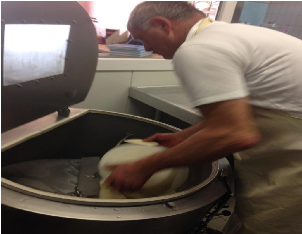
Figure 4. Werner Haase puts all the milk inside. After 10-20 Minutes he stops the machine, taking the liquids that have remained inside. In this case he takes it, transforming it into Buttermilk.
